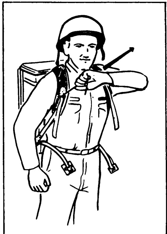
Figure 11. (1). Dismounting and emplacement of E8 launcher.
